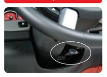
To adjust the steering wheel position, locate the adjustment lever under the steering column. Hold the steering wheel and rotate the lever down; then move the steering wheel to the desired position (the wheel can be adjusted up/down and in/out). Rotate the lever back up to lock the steering wheel in place.
